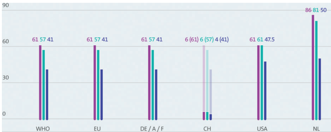
Figure 3: Recommended intensity limits in V/m and subsequent national legislation for the protection from electromagnetic radiation in the domain of mobile communication. Most countries base their national legislation on the recommendations of the ICNIRP (International Commission on Non-ionizing Radiation Protection). The Swiss NIS-Ordinance ( Verordnung über den Schutz vor nichtionisierender Strahlung ) fixes, however, two sets of limits: In light colors the so-called Exposure Limits ( Immissionsgrenzwerte ) and in dark colors the Installation Limits ( Anlagegrenzwerte ). This unique legislation procedure is based on the precautionary principle, as it is fixed in the Swiss Environmental act ( Umweltschutz-Gesetz ). Legend: magenta 2100 MHz or above; green 1800 MHz; blue 900 MHz.
