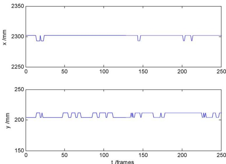
Fig. 2. Illustration of the 1-pixel limitation of variation of the recorded position when recording a stationary object:  $x$  and  $y$  position resulting from tracking a 10 s period where the animal was not moving.
