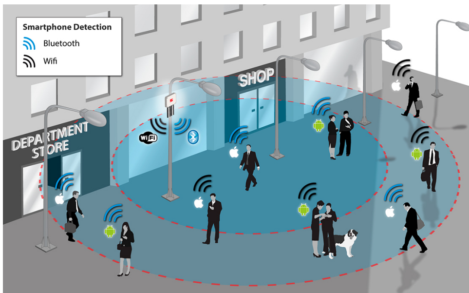
Fig. 2.3.: Combined Wi-Fi and Bluetooth tracking system
