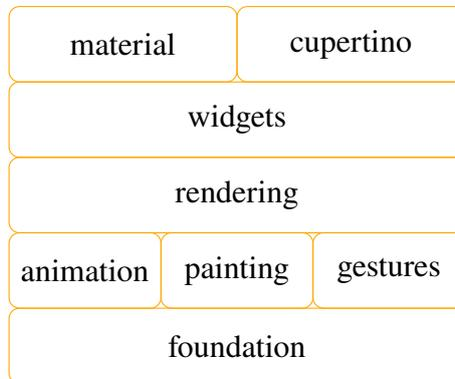
FIGURE 4.1 – Layers du Framework Flutter [7]
