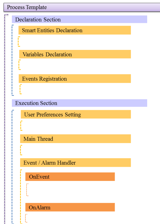
Figure 4.22: GPL4SRE elements structure
