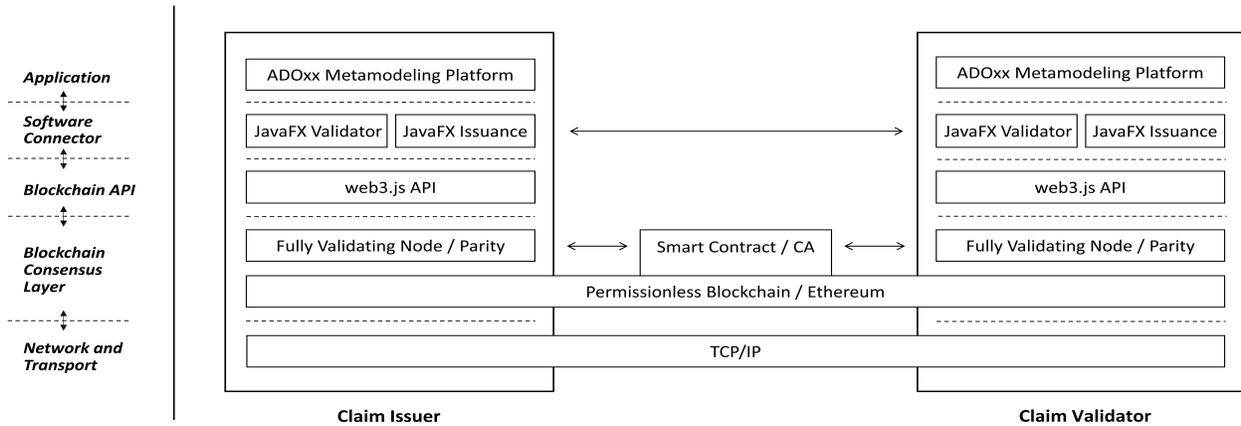
Fig. 2. Layered System Architecture Based on a Permissionless Blockchain for Communication
